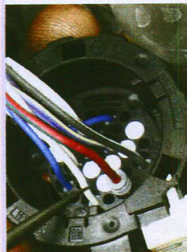
Check for unseated pin(s) in the transmission connector.
