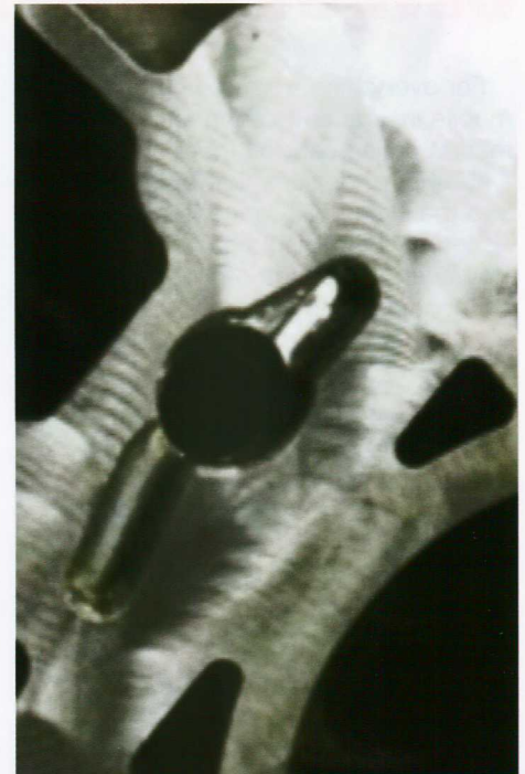
Abrasive discs can remove enough metal to cause leaks.
